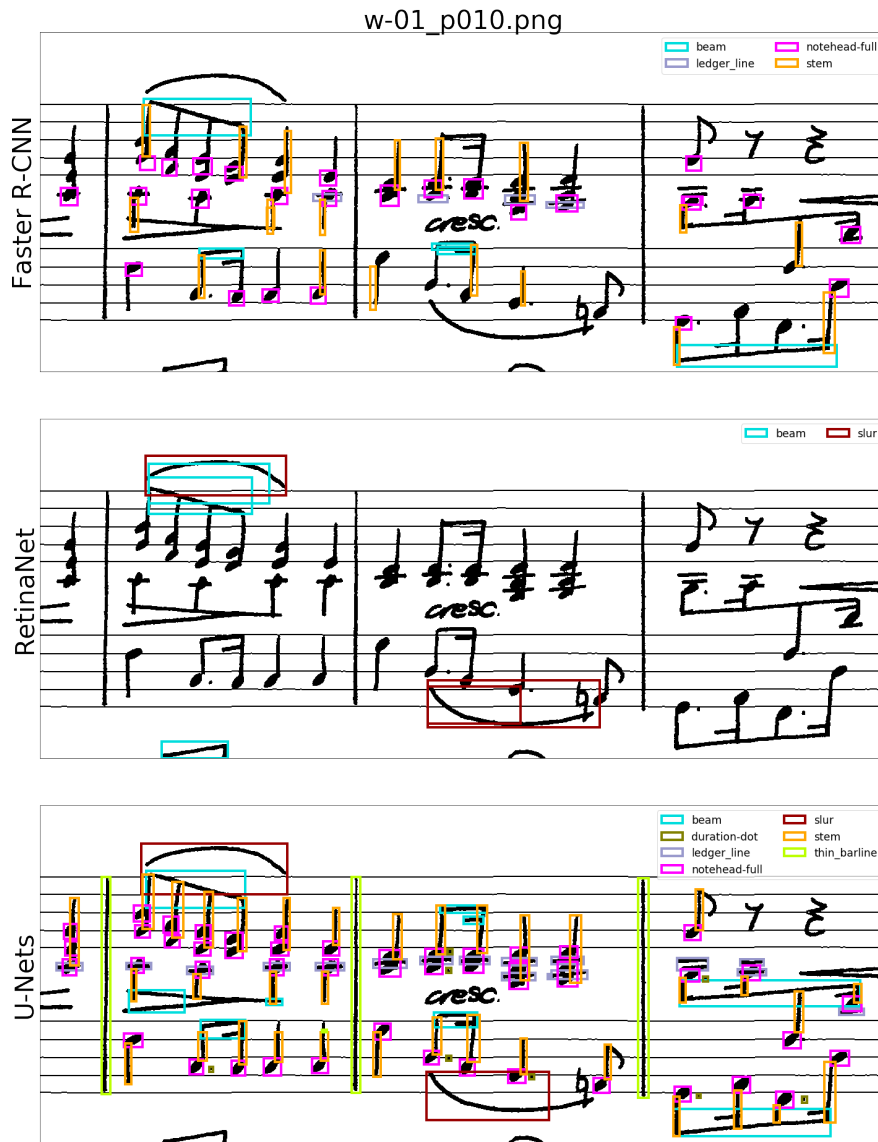
Figure 6. Detection sample on some selected classes from the MUSCIMA++ dataset. (top–bottom): Faster R-CNN, RetinaNet, and U-Nets detection results.
