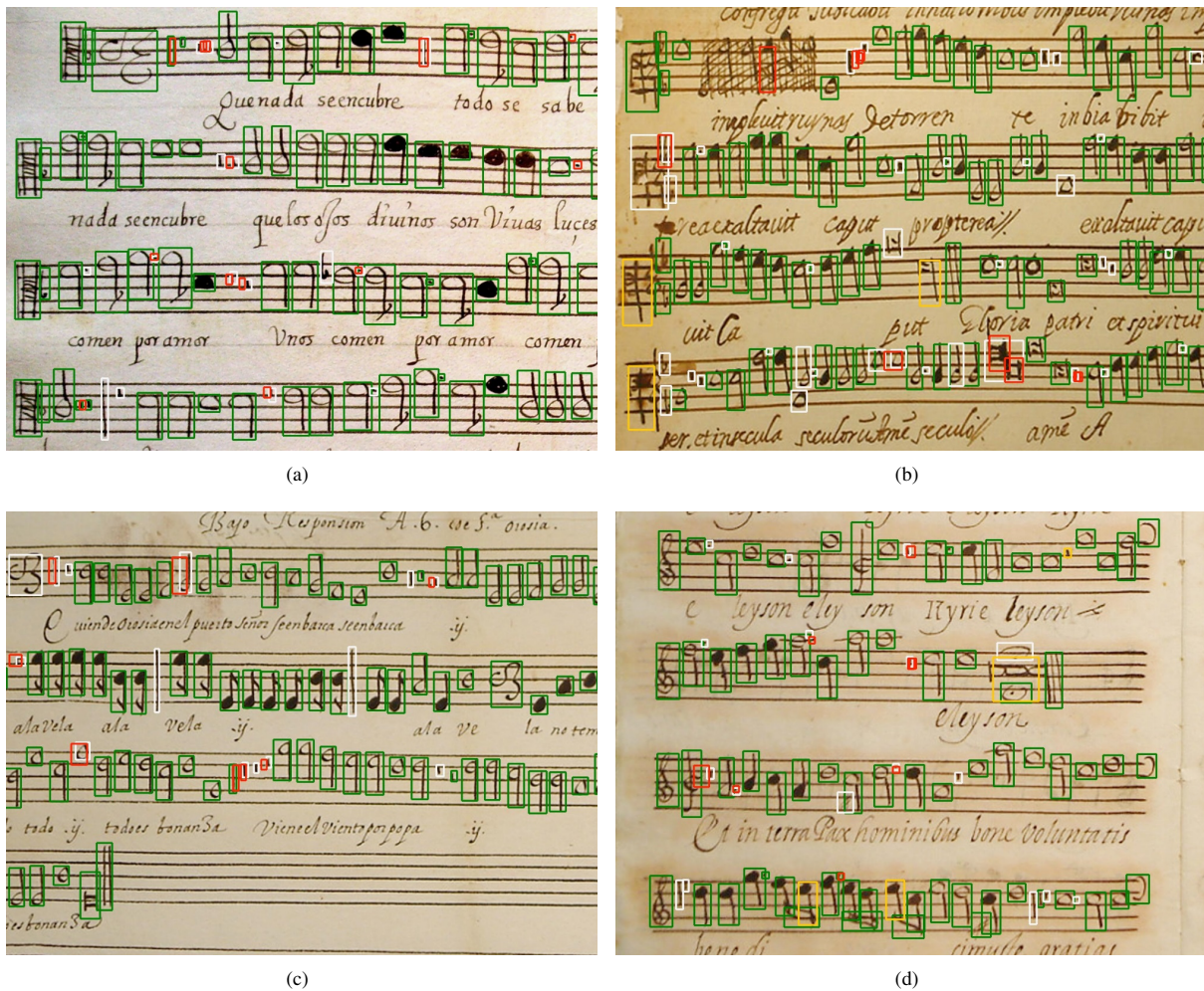
Figure 6. Visualization of the performance of the object detection stage with selected patches of the music documents: green boxes indicate true positive detections; white boxes are false negatives, that the network missed during detection; red boxes are false positive detections, where the model reported an object, although there is no ground-truth; yellow boxes are also false positives, where the bounding-box is valid, but the assigned class was incorrect.
