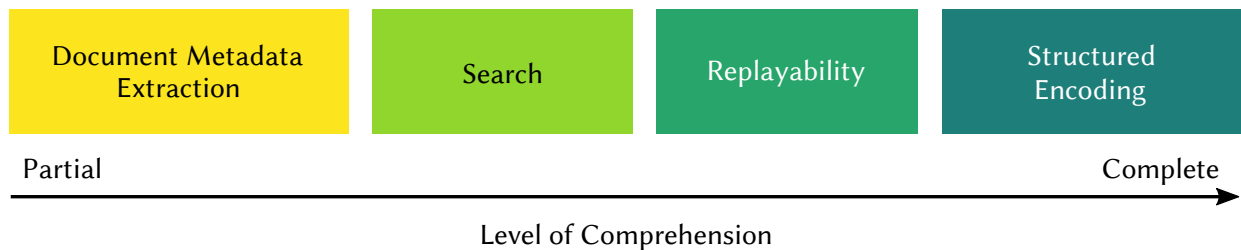
Fig. 13. Taxonomy of four categories of OMR applications that require an increasing level of comprehension, starting with metadata extraction where a minimal understanding might be sufficient, up to structured encoding that requires a complete understanding of music notation with all its intricacies.
